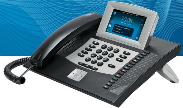
Android™-based hybrid VoIP telephone (SIP and IP system phone), with 4.3" colour touch display and preconfigured answering machine
